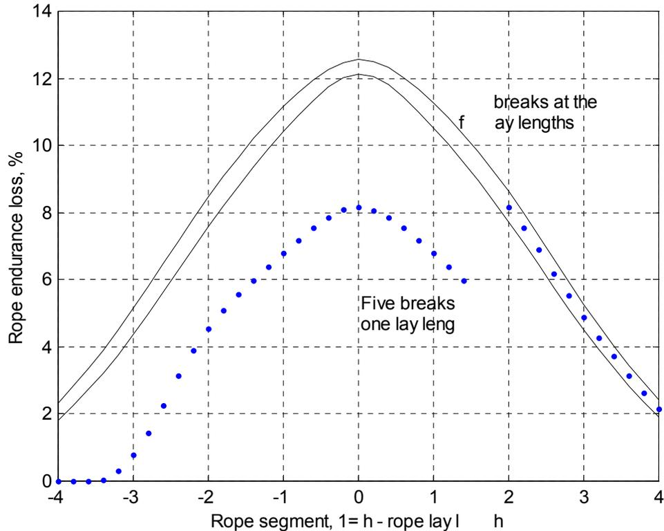
**Figure 3:** Statistical assessment of steel rope endurance loss due to wire breaks.
