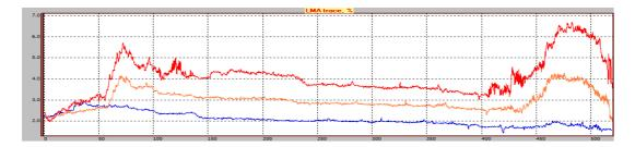
Figure 1 LMA-distributions of the shaft rope during three consecutive inspections
