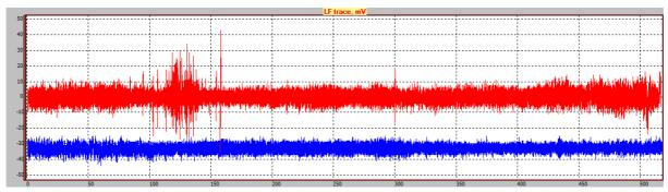
Figure 2. LF-distributions of the shaft rope for the 1st and 3d consecutive inspections
