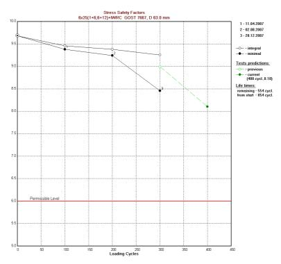
Figure 4. Degradation of safety factor of the shaft rope with operating time
