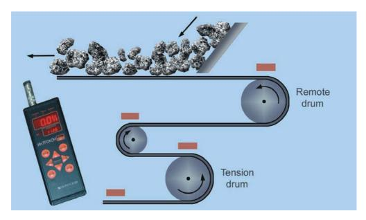
Fig. 2: Scheme of the scanner location on a conveyor.
