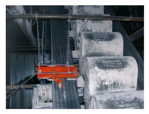
Fig. 6: The INTROCON scanner positioned on the Pocketlift conveyor belt.
