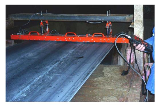
Fig. 1: INTROCON flaw detector on a conveyor.
