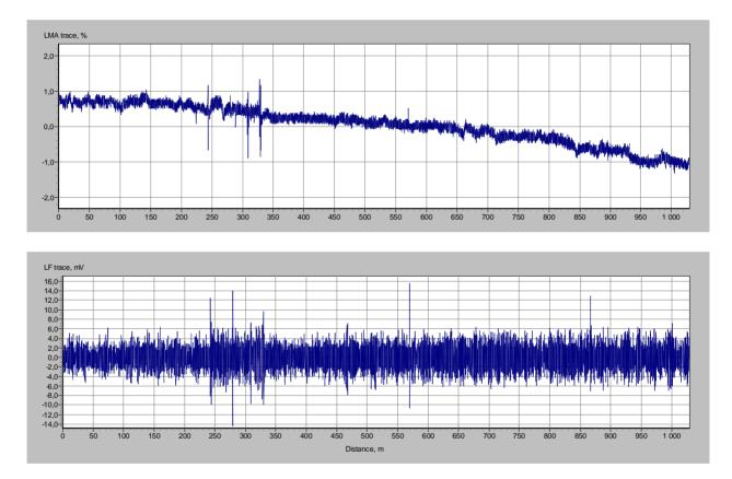
Fig. 6. LMA and LF charts of rope 38,5 mm. Charts obtained by INTROS rope tester.
