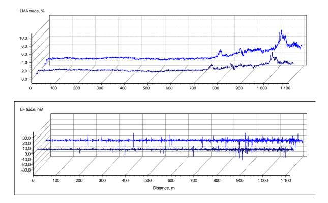
Fig.3. LMA and LF charts of brake rope 30,5 mm obtained by INTROS with 10 weeks interval
