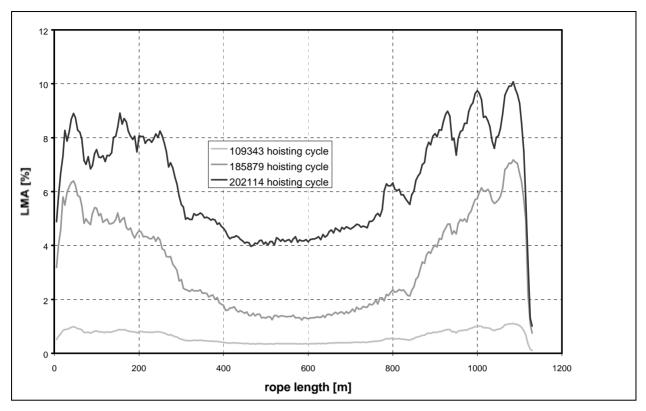
Fig. 4. LMA traces obtained from the rope after different hoisting cycles
