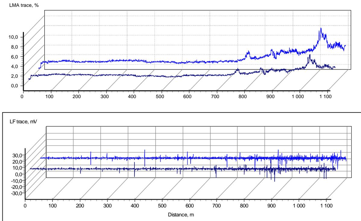
Fig.1. Charts of brake rope obtained by INTROS with 10 weeks time interval
