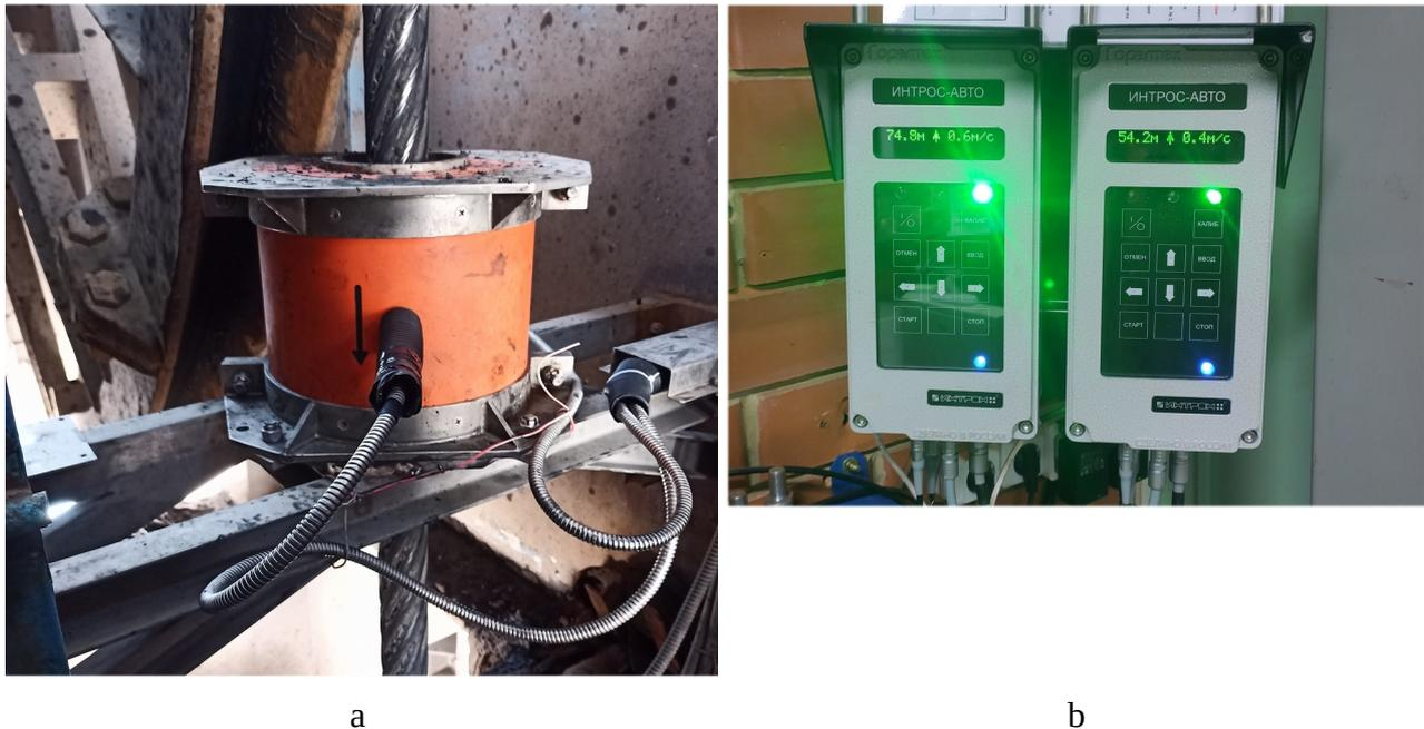
Figure. 1 Magnetic head (at mine hoist) and 2 control and display units of INTROS-AUTO at the double drum hoist
