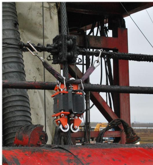
Figure 3. MH INTROS-AUTO at the rope of drilling rig hoist
