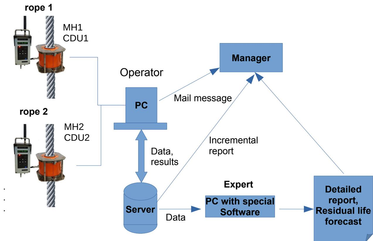
Figure 2. Data flow diagram for rope monitoring system
