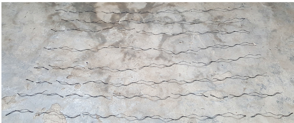
Figure 9. Broken wires of one strand after its unstranding.
