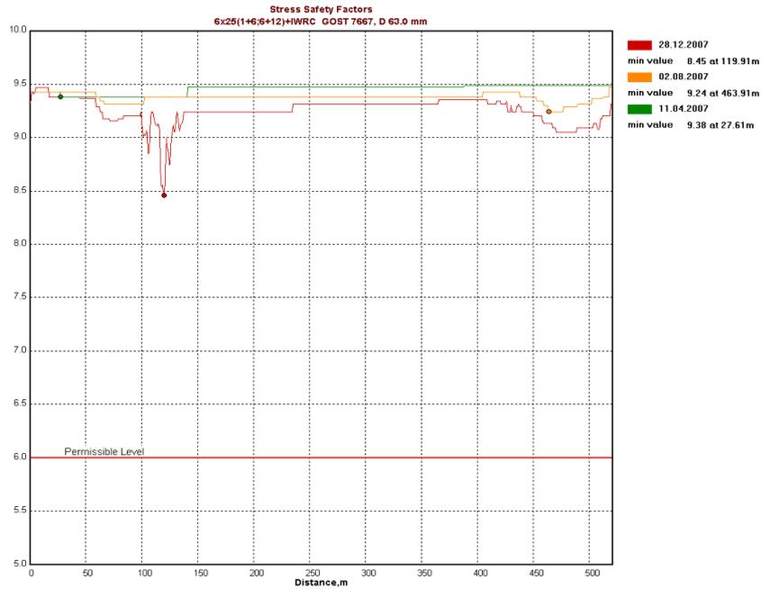
Figure 3. Distribution of safety factor of shaft rope during three consecutive inspections
