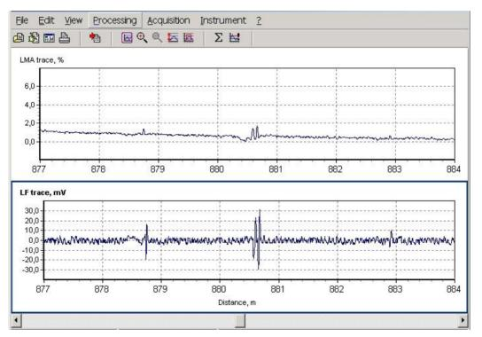
Figure 5. Part of data chart with 1+2+1 broken wires
