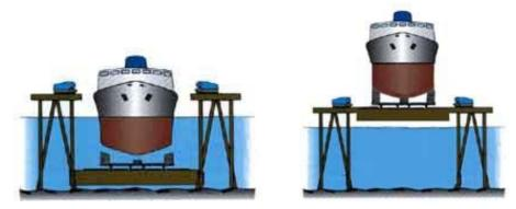
Figure 6. Scheme of the ship synchrolift
