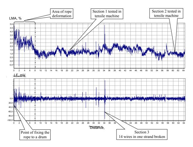
Figure 4: Data charts of the crawler crane DEK-251 boom rope (rope B).
