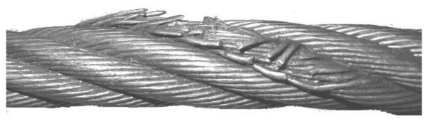
Figure 5: Wire breaks of the rope B one strand (section 3 in Figure 4).
